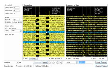
The illustration above is the unique Pulse-Ogram display in SignalVu-PC application license SVPH. This is a waterfall of triggered pulses showing their relationship to the trigger in time domain. Variations are immediately seen as changes in timing vs. trigger. Each time domain trace is represented as a spectrum on the right side of the display for immediate correlation of time and frequency domain effects.
