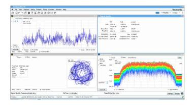
In the illustration above, a 5 GHz carrier modulated with 500 MSymbols/sec pi/4-QPSK is analyzed with the RSA7100B Option B800 and SignalVu-PC application license SVMH. A measurement summary, EVM vs. Time, and constellation display are shown along with the continuous monitoring of the DPX spectrum.
