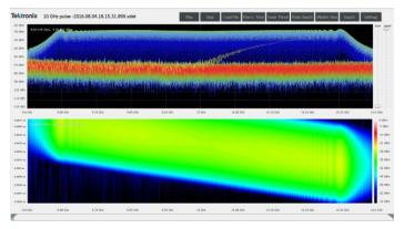
Above is a color-graded spectrum display combined with a 99% overlap spectrogram display as shown on DataVu-PC. You have full overlap/skip control to vary rate and detail of the streaming file for complete visualization of the data.
