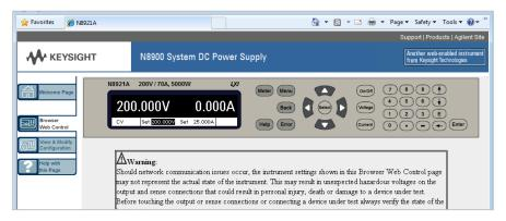
Figure 3. N8900 Series web graphical user interface for remote access and control of the power supply
