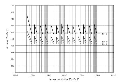
Figure 2. Accuracy of Cp and Cs when measurement frequency is 120 Hz (measurement range: 10 nF to 100  $\mu$ F / measurement signal level: 0.5 V)
