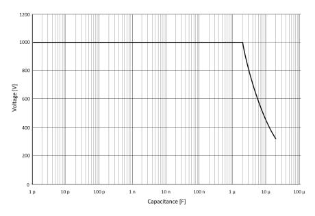
Figure 14. Maximum discharge withstands voltage (typical)
