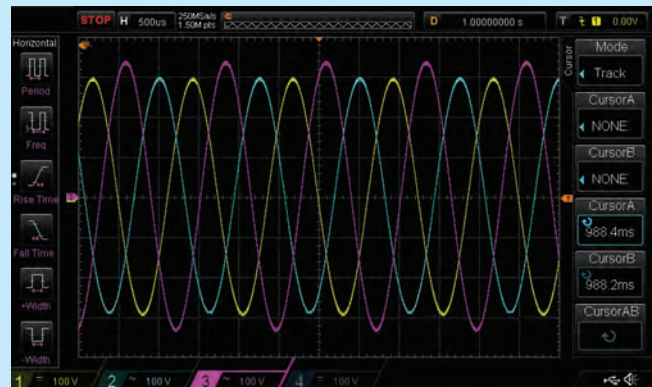
Three Phase Unbalance Voltage Test Captured
