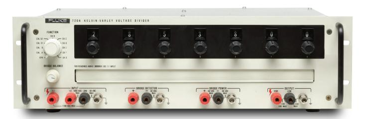
The 720A Kelvin-Varley Divider is a high-resolution primary ratio standard with absolute linearity of 0.1 ppm, temperature coefficient of linearity of 0.1 ppm/°C, and self-calibration capability.
